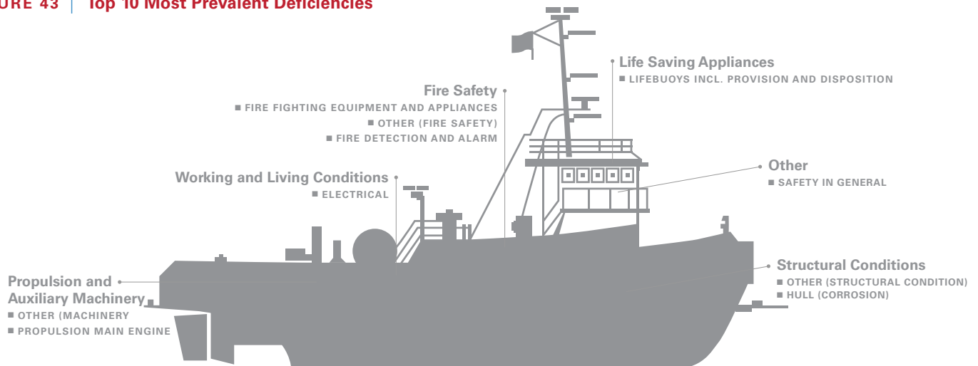
FIGURE 43 | Top 10 Most Prevalent Deficiencies
